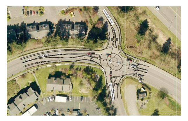
A rendering of the roundabout to be built along Reith Road at the intersection of Lake Fenwick Road and 44th Avenue South. COURTESY IMAGE, City of Kent
